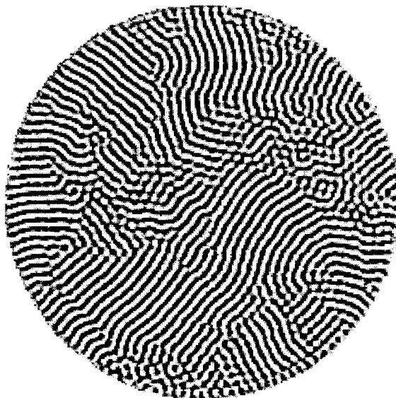
Figure 41 An example of the Küppers-Lortz unstable rolls for \Omega = 15.4 and \text{CO}_2 at a pressure of 32 bar with \sigma = 1.0 and \varepsilon = 0.05 . After Hu et al (1995b).
